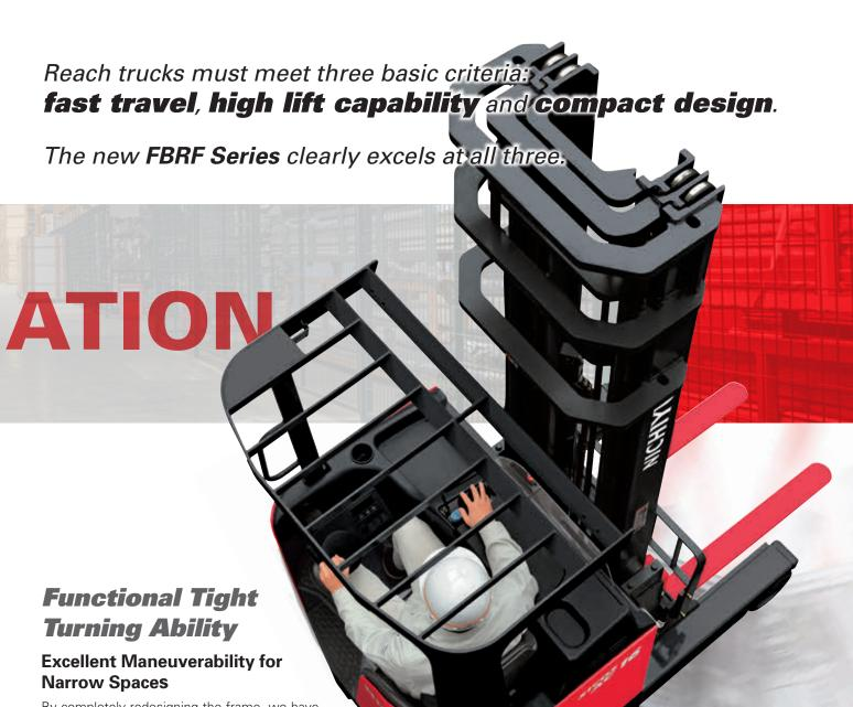
By completely redesigning the frame, we have reduced the minimum turning radius and right angle stacking aisle width. As a joint result with newly adopted 360° endless steering, we now lead the industry in space efficiency.
